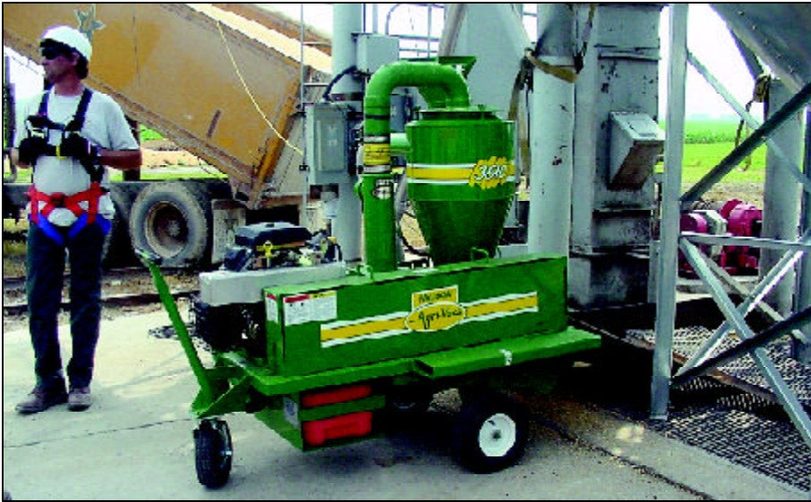
A pneumatic conveying system such as this Walinga Agri-Vac can be an important tool in extracting victims entrapped in grain.
