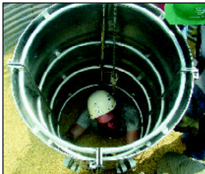
The use of a metal cofferdam prevents additional grain from cascading down onto entrapped victims and relieves pressure from grain during the rescue.
